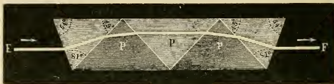
FIG. 178.—Direct Vision Prism.
